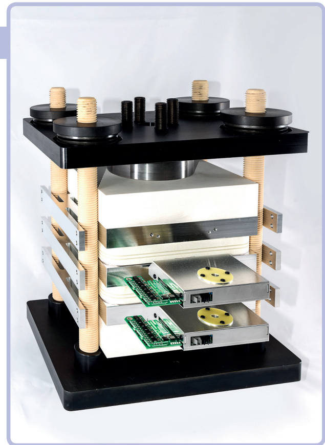
Example of stack with 5SNA3000K452300 IGBT modules
